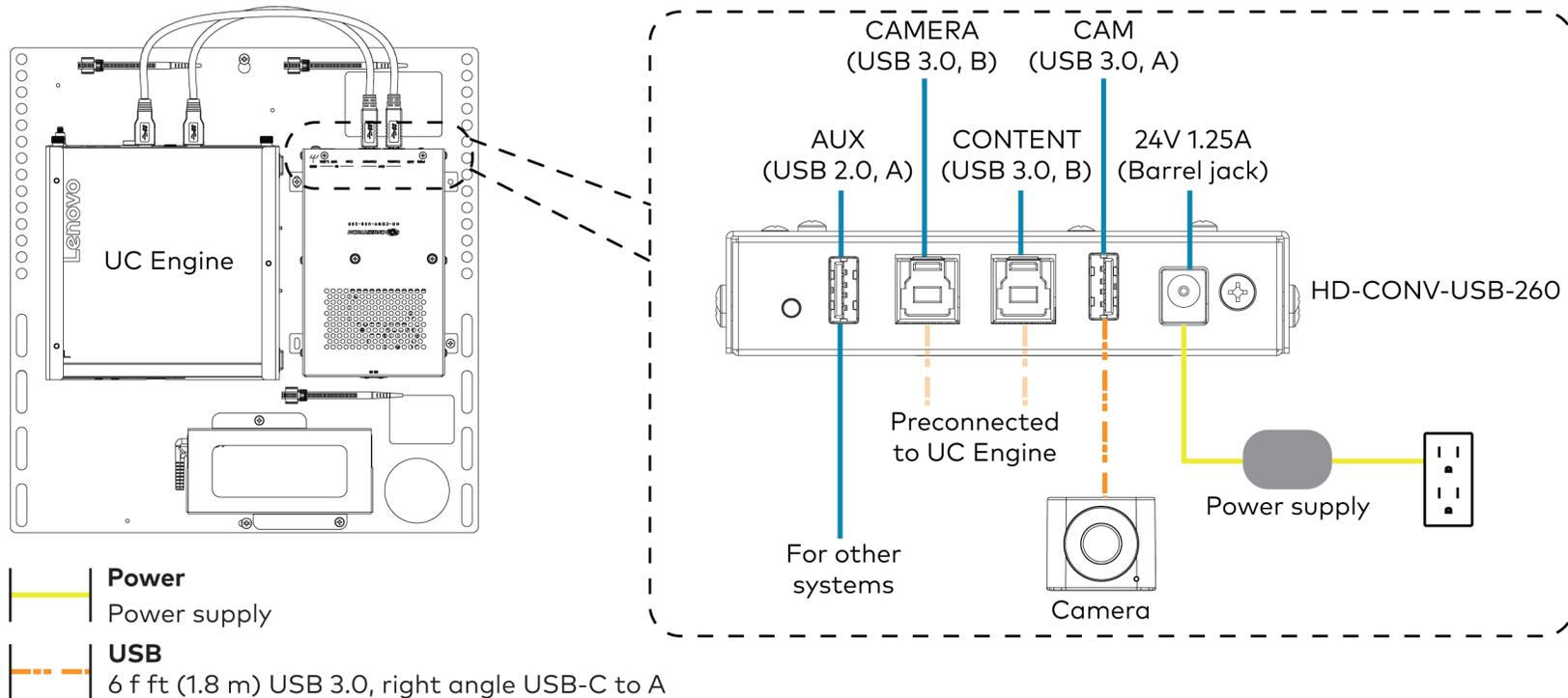
5. Bundle the cables to the bracket assembly with the integrated cable tie wraps. The cable tie wraps are reusable.
