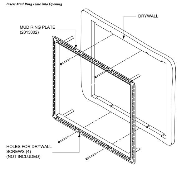
**NOTE** SCREW LENGTH SHOULD NOT EXCEED DRYWALL THICKNESS BY MORE THAN 1/2" (12.7 MM).
