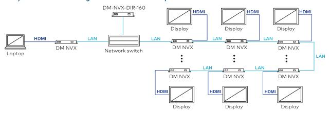
Due to limited bandwidth for audio and video, a USB host or device on a daisy chained endpoint is not recommended. For maximum flexibility and the ability to reconfigure video walls with multiple sources, connect DM NVX endpoints directly to switches rather than daisy chain the endpoints.
