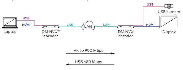
An encoder that attempts to send 900 Mbps video and 480 Mbps USB 2.0 traffic exceeds the maximum network link bandwidth of 1 Gbps and, as a result, the link will fail.
