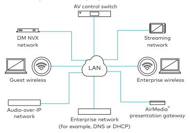
Consideration must be given to blocking at both the switch level and the network design level. DM NVX network switches must have enough switch fabric bandwidth to support full nonblocking bidirectional gigabit bandwidth on all ports simultaneously. This is a common feature in enterprise-grade gigabit network switches, but it should not be assumed that a switch is nonblocking or is configured as nonblocking.
