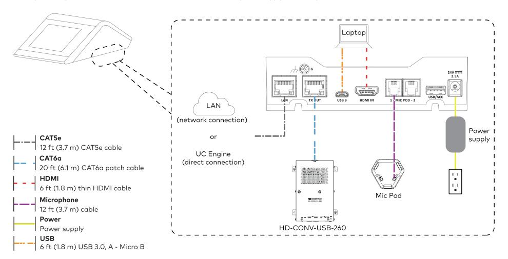
3. Connect the power supply and camera to the bottom of the content ingest device (HD-CONV-USB-260). Connect the power supplies to an AC power outlet.
