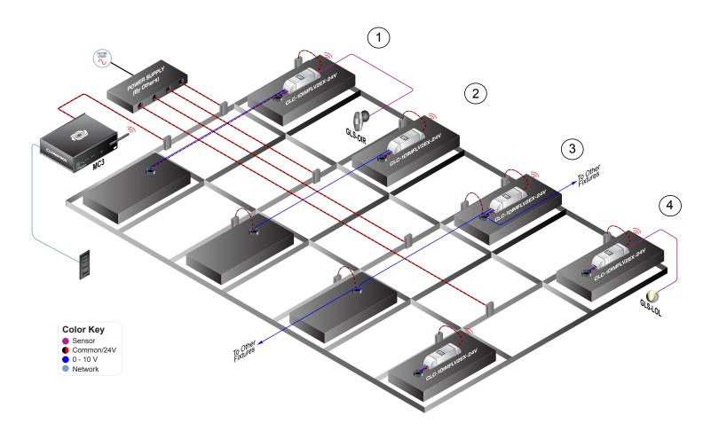
This diagram illustrates multiple ways of applying the CLC-1DIMFLV2EX-24V. Each row of lighting, identified by its number, is configured differently. Each method has value in certain applications.
