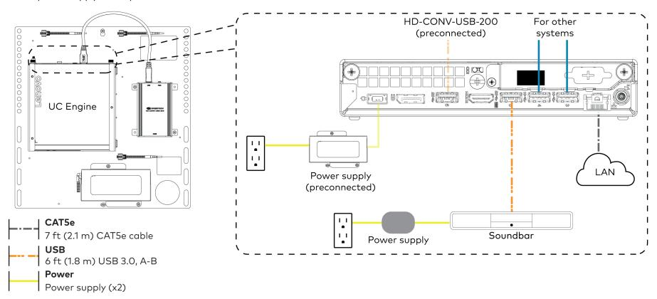
3. Connect displays to the UC Engine.
