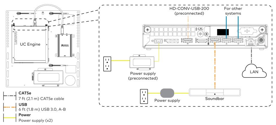
3. Connect displays to the UC Engine.
