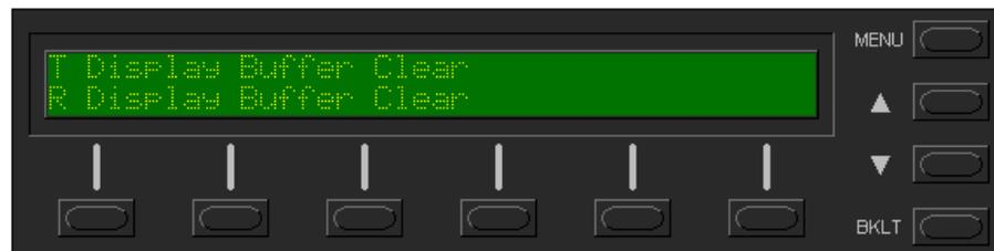
The top line of the T/R screen displays data that is transmitted out the selected ports in the selected format. The bottom line displays the data that is received in the selected format. If more data is present in the display buffer, only the most recent data is displayed (older data scrolls off the screen).
