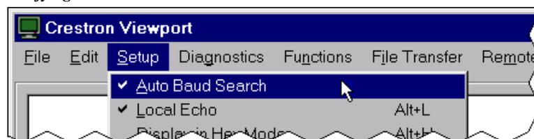
6. While the Viewport is displayed, select **Setup | Communications settings** (alternatively, depress **Alt+D**) to open the "Port Settings" dialog box. Refer to the illustration on the next page.
