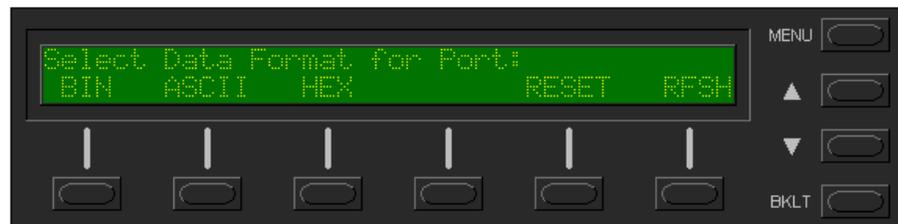
Since there is no room on the T/R screen for button text, RESET and RFSH (refresh) are provided on the Format Selection Menu to show their location on the T/R screen.
