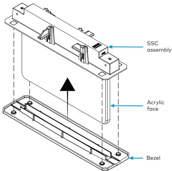
4. Slide the bezel retained during the disassembly carefully over the acrylic face until the magnets on the bezel snap into place against the SSC assembly.
