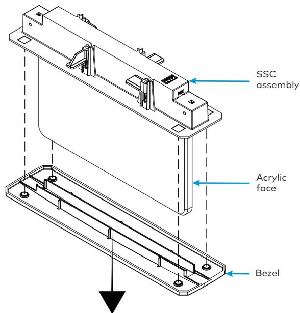
1. Remove the bezel from the SSC assembly by gently pulling it away from the installed sign to break the magnetic hold, then sliding it down and across the acrylic face. Retain the bezel.
