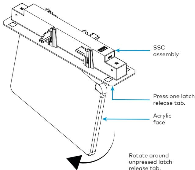
2. Use both hands to complete the following items simultaneously and remove the acrylic face from the SSC assembly.
