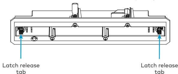
**NOTE:** Each end of the SSC assembly has a latch release tab that secures the acrylic face to the assembly.
