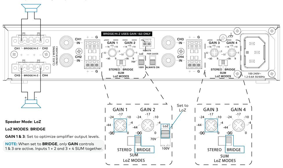
2 Channel x up to 150 W Bridged Output (High Impedance)
