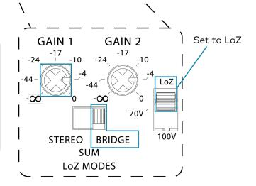
1 Channel x up to 300 W Bridged Output (High Impedance)
