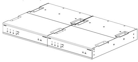
2. Use a Phillips screwdriver to gang the amplifiers together with two of the included joining plates and the eight included  $8-32 \times 5/16$  in. screws.
