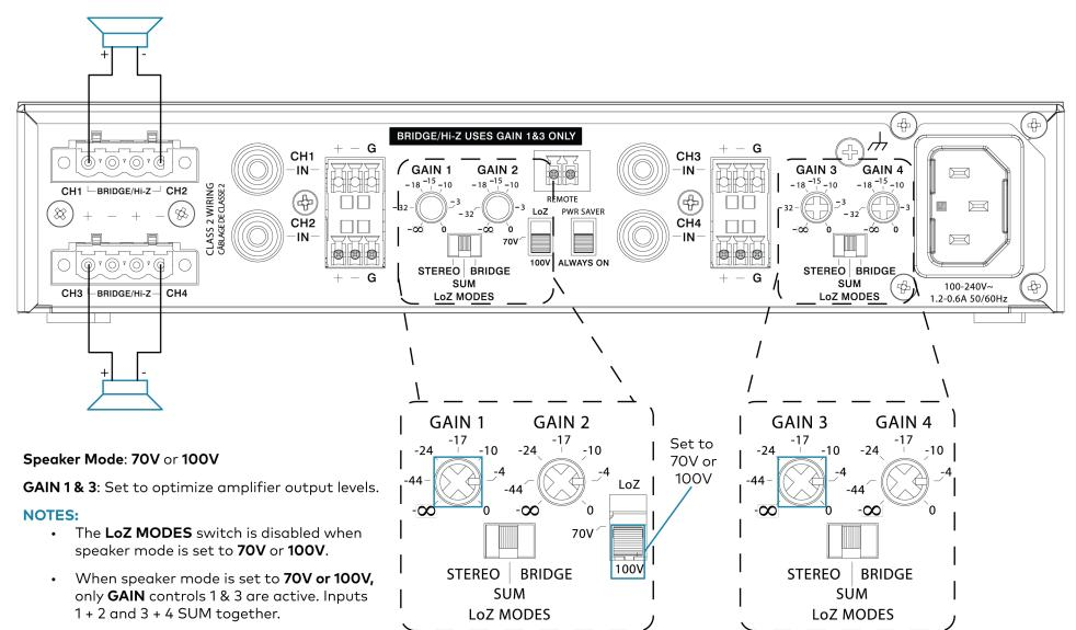
1 Channel x up to 300 W Bridged Output (Low Impedance)
