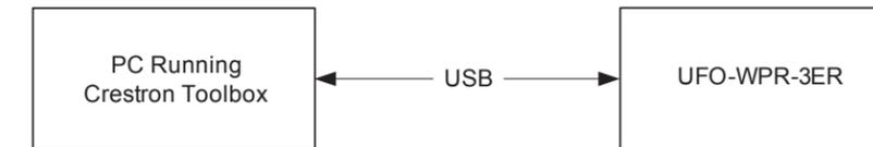
The USB port on the UFO-WPR-3ER's included UFO-WPR-3ER-DS docking station connects to the USB port on the PC via the included Type A to Type B USB cable:
