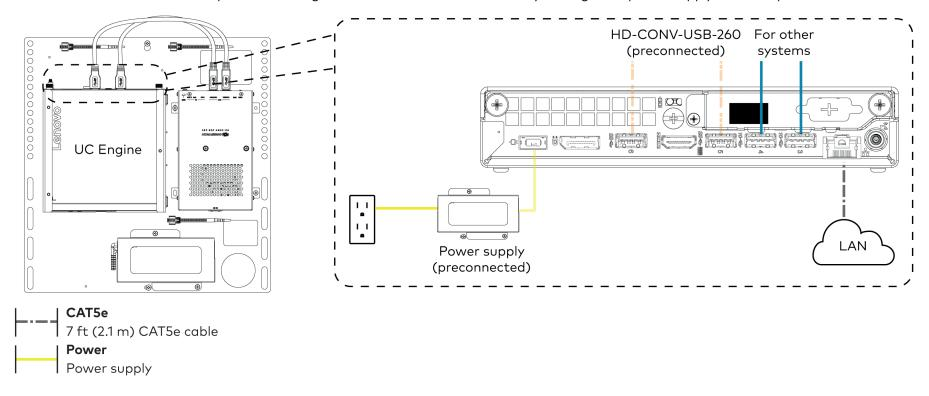
3. Connect displays to the UC Engine.
