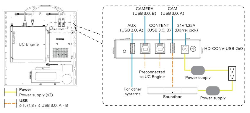
5. Connect power and the content ingest device (HD-CONV-USB-260) to the top of the UC Presentation Transmitter. Connect the UC Engine or LAN to make a direct or network connection as described in step 1.
