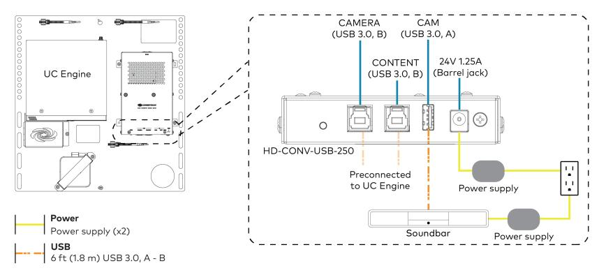
3. Connect power and the content ingest device (HD-CONV-USB-250) to the top of the UC Presentation Transmitter. Connect the UC Engine or LAN to make a direct or network connection as described in step 1.
