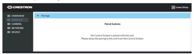
Pair the CCS-WB-1 with a control system from the CCS-WB-1's SIMPL programming module that is part of a SIMPL Windows program. For details on pairing and the SIMPL programming module, refer to the module's help file.
