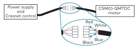
Cresnet QMT Shade Motor with the Power and Control Coming from Separate Sources
