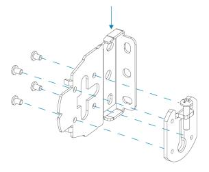
Reassemble the bracket. Ensure the keyhole is parallel with the wall when it is mounted.
