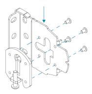
Reassemble the bracket. Ensure the keyhole is parallel with the wall when it is mounted.
