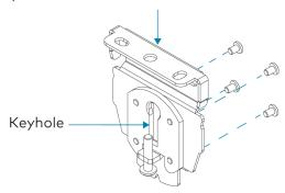
Rotate Keyhole: Right-Side Wall Mount to Left Side Wall Mount
