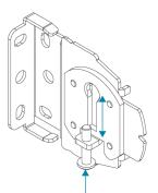
Tighten or loosen the screw to level the shade.
