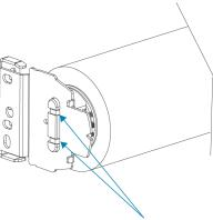
Maneuver the motor end into the bracket slot.
