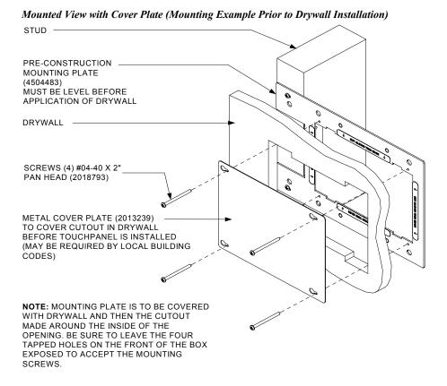
**NOTE:** The four tapped holes on the front of the mounting plate must be exposed to accept the touchpanel mounting screws. These holes are found beneath the drywall just outside the four corners of the opening made by cutting out the drywall. Refer to the **NOTE** in "Mounted View with Cover Plate" illustration above.
