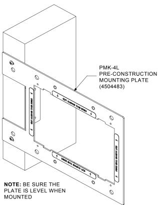
CAUTION: Allow an air gap of at least 12 inches (30.48 cm) in the wall cavity above and below the touchpanel for heat dissipation.
