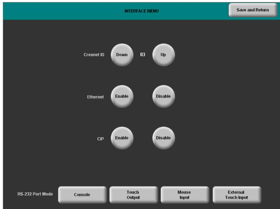
Two buttons adjacent to the Cresnet ID and its displayed hexadecimal number, **Down** and **Up**, decrease and increase the Cresnet ID by one, respectively.
