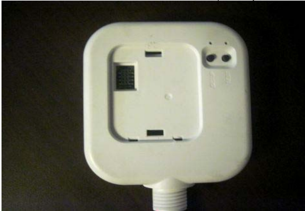
Photo 2 - Exterior view of ZUMMESH-JBOX series models (accessory dock cover removed)
