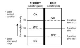
\* If the switch is set within the stable range, the reliability against changes in ambient conditions (temperature, voltage, dust, shift of setting, etc.) increases. Be careful of changes in the ambient conditions for which a stable range cannot be obtained.
