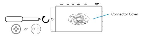
**NOTE:** For additional security, replace the screws with the included spanner screws. A 1/4 in. bit is supplied to install the spanner screws.
