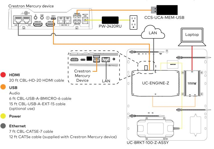
3. Connect the display devices and camera to the UC-ENGINE-Z as shown below.
