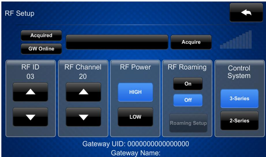
4. Tap **Acquire** to place the TST-902 into Acquire mode. An "Acquire in progress" message is displayed on the RF Setup screen, and the TST-902 will be acquired by the ER gateway within two minutes.
