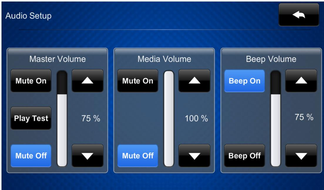
Use the **Audio Setup** screen to control the main volume, media volume, and beep volume settings for the touch screen.
