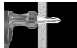
c. Insert the included anchor key to pop the anchor open and lock it behind a hollow wall.
