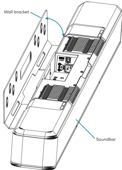
6. Place the wall bracket over the screws, and hand tighten the screws until the wall bracket is secured to the wall.
