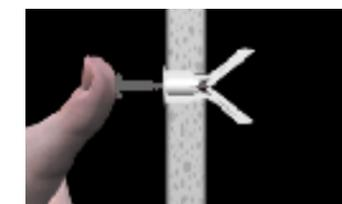
d. Drive the screw part of the way into the anchor, leaving approximately 1/4 in. of the screw exposed.
