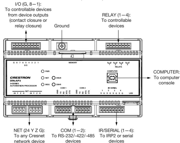
*Hardware Connections for the DIN-AP3 (Bottom View)*
