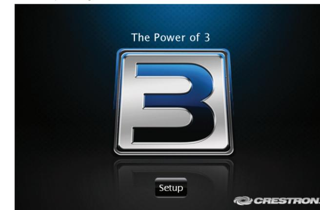
3. Click **Setup** to display the DIN-AP3 setup menu. The DIN-AP3 **Setup** menu displays the IP address, hostname, and MAC address of the device. The screen also allows access to various setup and programming screens.
