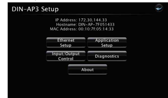
4. From the DIN-AP3's **Setup** menu, click the following options to configure the control system:
