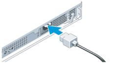
8. Secure the power cable to avoid tangled wires and possible disconnection.
