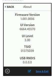
Use the **About** screen to view information about the TSR-310, including the loaded firmware, the operating system versions, and the device RNDIS address (if the TSR-310 is connected to a computer via USB).
