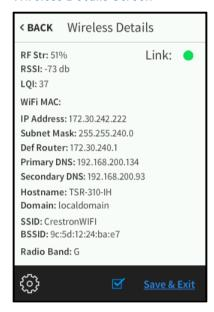
Use the **Wireless Details** screen to view various wireless connection details for the TSR-310 and the current WAP. A **Link** indicator is also provided to indicate the status of the wireless connection. (Green indicates that the wireless connection is active.)
