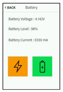
Use the **Battery** screen to view the TSR-310 battery voltage, charge, and current levels.
