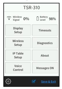
The setup screen provides buttons for the display setup, wireless setup, IP table setup, voice control, standby timeouts, and diagnostics. There is also a button to toggle system messages on or off and an **About** button that provides information about the TSR-310.
