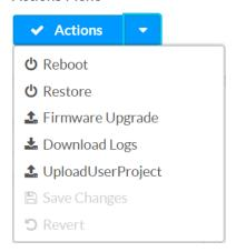
Once any changes have been made to the TSR-310 configuration, the **Actions** button changes to a **Save Changes** button. Click **Save Changes** to save changes to the configuration settings.
