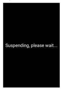
During a suspend test, the TSR-310 enters suspend mode. To exit suspend mode, pick up the TSR-310, tap any of the hard buttons, or touch the LCD display. The TSR-310 wakes and returns to the **Diagnostics** screen.
