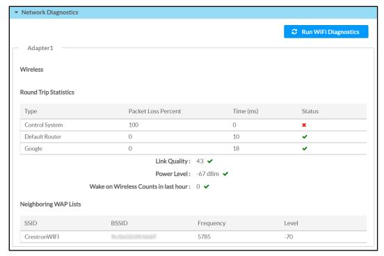
Click **Run Wi-Fi Diagnostics** at the top of the page to run a diagnostic test for the Wi-Fi connection. Once the diagnostic test has completed, the configuration utility refreshes to display the current values for the connection data.
