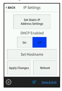
Use the **IP Settings** screen to configure IP, DHCP (dynamic host configuration protocol), and hostname settings for the TSR-310.
