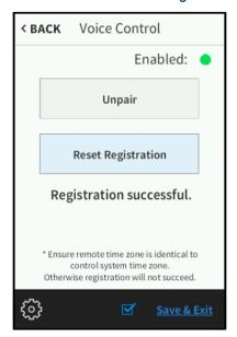
**NOTE:** If a registration error displays, ensure that the TSR-310 is connected to the control system over IP, the control system is connected to the voice services provider, the voice registration program is running and has been programmed correctly, and the time zone has been set correctly. For more information, refer to "Appendix B: Set Up Voice Control Services," starting on page 49.
