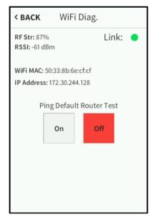
Use the **Wi-Fi Diag.** screen to view and test the Wi-Fi network connection. The **Wi-Fi Diag.** screen displays the Wi-Fi connection RF strength, RSSI (received signal strength indication), MAC address, and IP address. A **Link** indicator is also provided to indicate the status of the Wi-Fi connection. (Green indicates that the Wi-Fi connection is active.)
