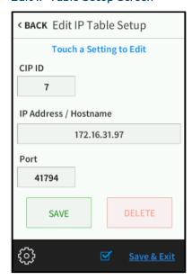
Tap the CIP ID text field to display the on-screen hex keypad.
