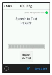
Use the **MIC Diag.** screen to test the TSR-310 built-in microphone and the voice recognition feature. A **Voice Recognition Link** indicator is also provided to indicate the status of the voice recognition feature. (Green indicates that the feature is active.)
