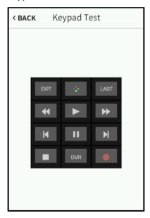
Pressing any of the buttons shown in the first **Keypad Test** screen switches the screen back to displaying the upper buttons.
