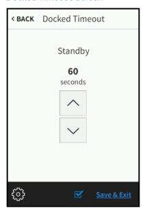
Tap the up and down arrows to increase or decrease the standby timeout duration when the TSR-310 is docked from 0 to 120 seconds.
