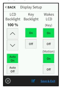
Use the **Display Setup** screen to adjust LCD backlight and hard button backlight settings:
