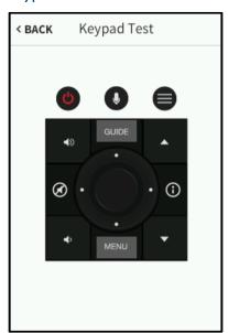
Use the **Keypad Test** screen to test the functionality of the remote buttons. When one of the buttons is pressed, its respective indicator lights on the screen.
