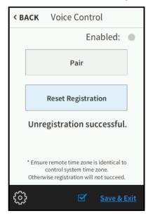
Tap **Reset Registration** to force the TSR-310 to clear all local registration information. Use this function only if the TSR-310 is unable to register or unregister successfully.
