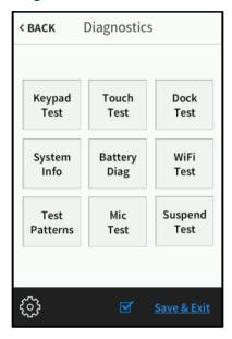
Use the **Diagnostics** screen to access various diagnostic test screens for the TSR-310. Each test screen is described in the sections that follow.
