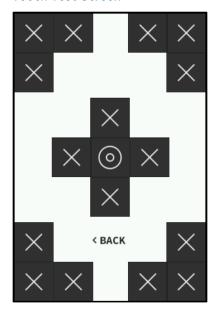
Use the touch test screen to test the touch functionality of the display. When a location button is tapped, its respective indicator lights on the screen.
