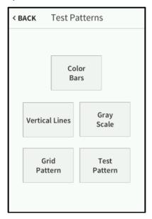
Use the **Test Patterns** screen to display any of the available test patterns. Tap one of the buttons on the screen to load its respective test pattern.
