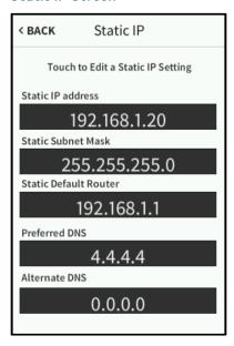
To edit the static IP address, the static subnet mask address, the default router address, and the preferred and alternate DNS addresses, tap the text field underneath the setting name. An on-screen keypad is displayed.
