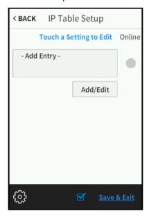
Use the **IP Table Setup** screen to view and edit the IP table settings for connecting the TSR-310 to a control system. The **IP Table Setup** screen also provides an **Online** indicator for the IP table entry. (Green indicates that the control system is online.)
