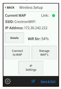
Use the **Wireless Setup** screen to view wireless connection details, to connect to a WAP, to manage existing WAPs, and to configure IP settings.
