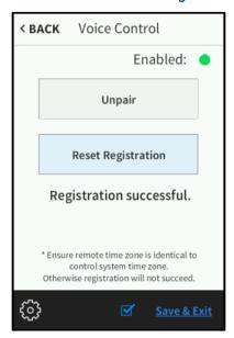
**NOTE:** If a registration error displays, ensure that the TSR-310 is connected to the control system over IP, that the control system is connected to the voice services provider, that the voice registration program is running and has been programmed correctly, and that the time zone has been set correctly.
