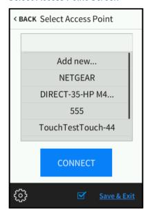
Use the **Select Access Point** screen to connect the TSR-310 to an existing WAP that is in range or to configure a new WAP.
