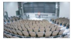
The tracking shot moves to and zooms into the area where motion has occurred. As it is zooming in toward the position defined in Preset 1, the full-room view shows a red box around the presenter's face once it has been detected.
