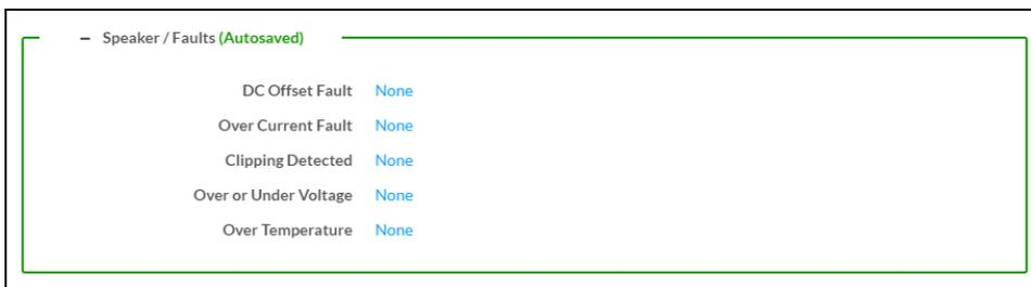
The Speaker/Faults section is a read-only field that displays the status of the **DC Offset Fault**, **Over Current Fault**, **Clipping Detected**, **Over or Under Voltage**, and **Over Temperature** detectors for the zone output. If clipping or a given fault type is detected, then its corresponding readout displays **Fault Detected** in red. Otherwise, it displays **None** in blue.
