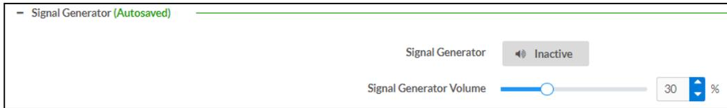
The DM-NAX-BTIO-1G has a built-in signal generator that allows an integrator to send an audio signal to the output to test functionality.
