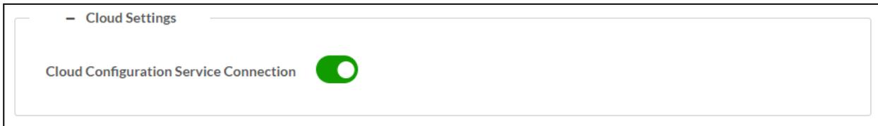
Set the **Cloud Settings** toggle to enabled (right) or disabled (left) to specify whether the DM-NAX-AUD-USB can communicate with the XiO Cloud® platform.
