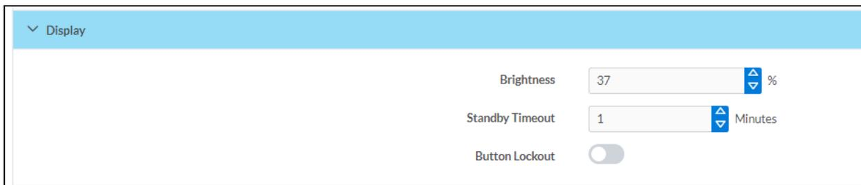
The **Display** section contains settings that affect the front panel OLED display of the DM-NAX-BTIO-1G.
