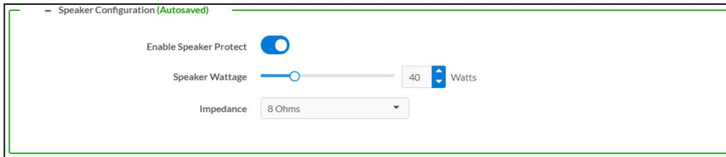
1. Set the **Enable Speaker Protect** toggle to the right position to enable speaker protection for the zone output. Set the toggle to the left position to disable speaker protection. By default, **Enable Speaker Protect** is set to the left position.
