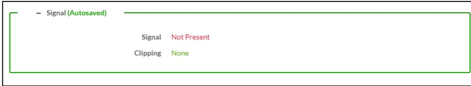
The **Signal** section is a read-only field that displays the **Signal** and **Clipping** status of the zone output.
