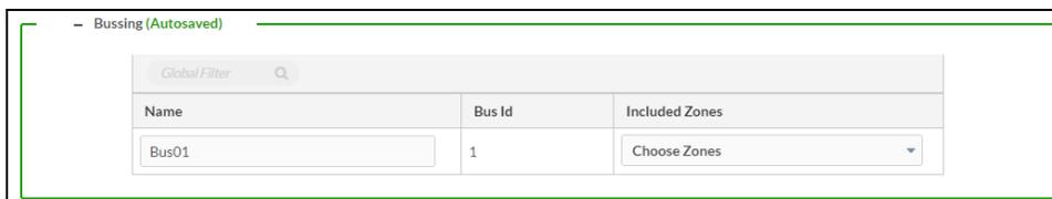
The bussing feature on DM NAX devices allows an integrator to assign any number of selected zones to a fixed group of zones (bus). Zones in a bus track the other zones' volume and routing. For example,
