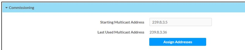
Select **Assign Addresses** to give each DM NAX transmitter in the DM-NAX-16AIN a unique multicast address beginning with the specified **Starting Multicast Address**. The valid range for **Starting Multicast Address** is 239.8.0.0 to 239.255.255.239.
