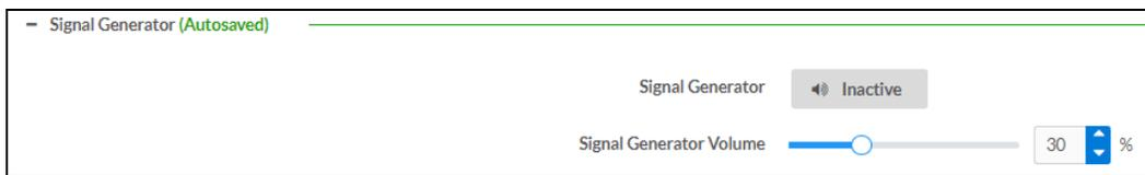
The DM-NAX-AMP-X300 has a built-in signal generator that allows an integrator to send an audio signal to any number of selected zones to test output functionality.
