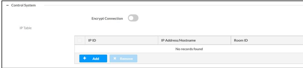
1. Set the **Encrypt Connection** toggle to the right to enable a secure connection between the control system and the DM-NAX-16AIN. Set the toggle to the left to use an unencrypted connection to the control system. If the toggle is set to the right:
