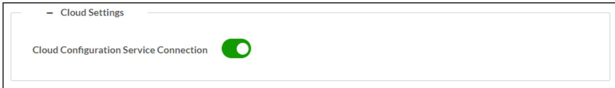
Set the **Cloud Settings** toggle to enabled (right) or disabled (left) to specify whether the DM-NAX-AUD-IO can communicate with the XiO Cloud® platform.
