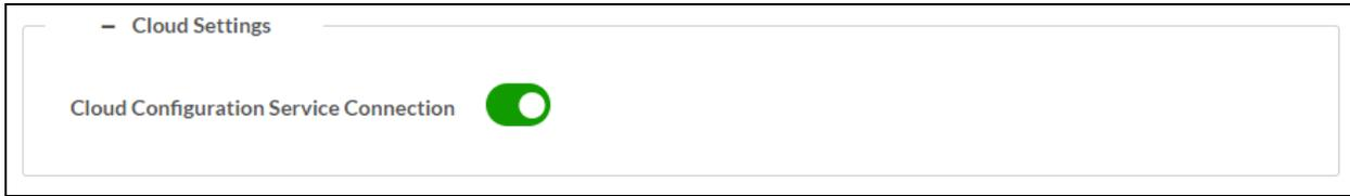
Set the **Cloud Settings** toggle to enabled (right) or disabled (left) to specify whether the DM-NAX-2XLRI-1G can communicate with the XiO Cloud® platform.
