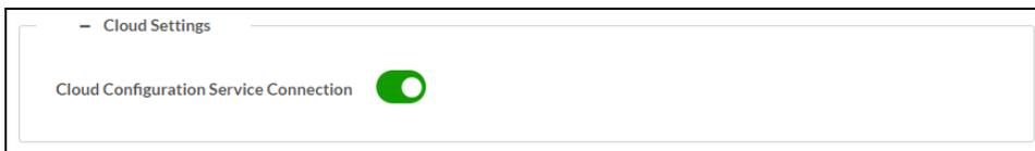
Set the **Cloud Settings** toggle to enabled (right) or disabled (left) to specify whether the DM-NAX-AMP-X300 can communicate with the XiO Cloud® platform.
