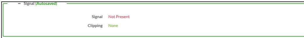
The **Signal** section is a read-only field that displays the **Signal** and **Clipping** status of the zone output.
