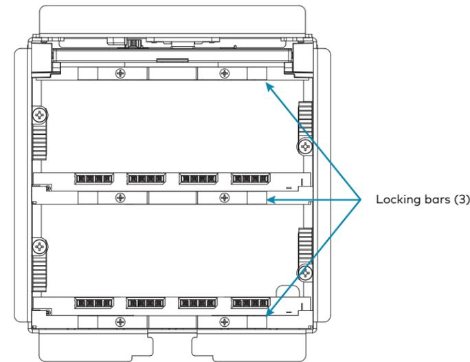
4. Lift and remove the modules to be replaced.
