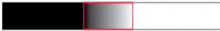
Fig 2: The dynamic range (shown in red) captured with WDR OFF. The area to the left is underexposed, and the area to the right is overexposed.
