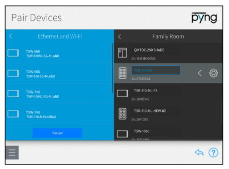
Once the TSR-310 has been paired with the system and added to a room, the Performance UI operational screens may be accessed from the TSR-310 touch screen display.
