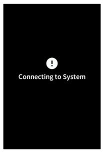
This alert is closed automatically once a connection to the CP3-R is established. If this message is displayed for a prolonged period, check the connection to the CP3-R.
