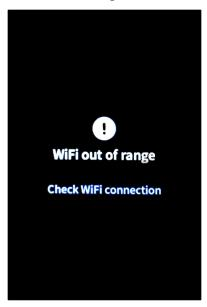
This alert is closed automatically once the TSR-310 is back in range of the wireless access point. If this message is displayed while in range of the access point, ensure that the access point is powered on and is functioning properly.
