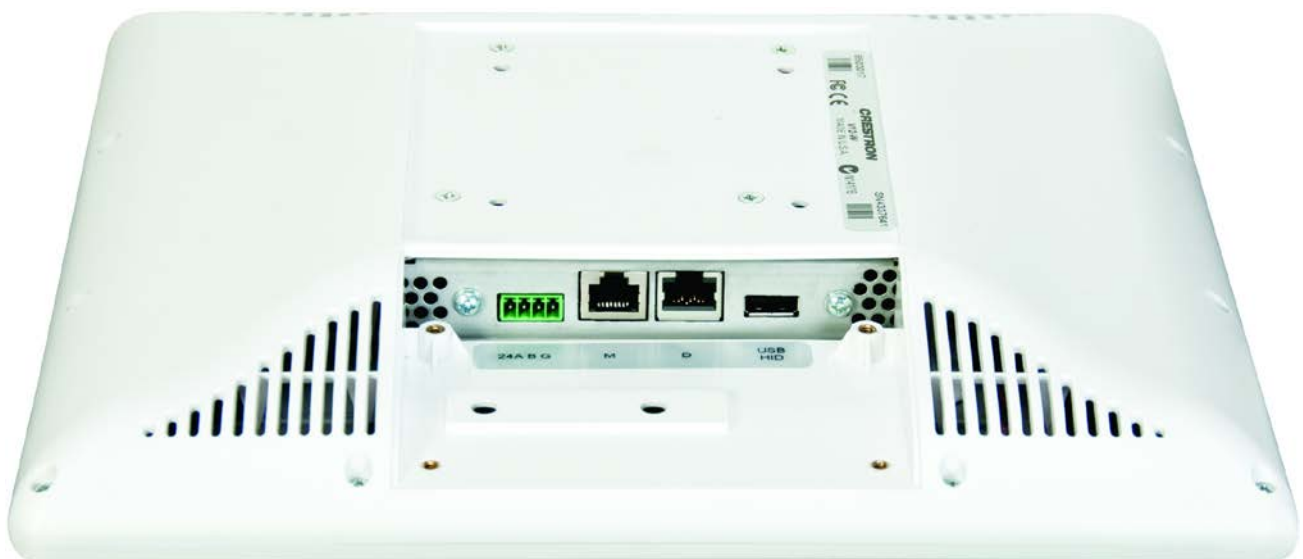
V-Panel Physical View (Rear Showing Connector Ports)
