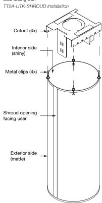
Confirm that all cables are surrounded by the shroud before joining the two strips of hook and loop fabric fasteners at the opening.
