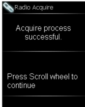
5. Press the scroll wheel to take the MLX-3N out of *Acquire* mode and return to the “Radio Options” screen. Press the “MenuBack” button to exit from the “Radio Options” screen.
