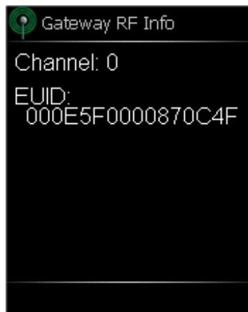
The “Gateway RF Info” screen shows the gateway’s channel and EUID. Press the “MenuBack” button to return to the “Radio Information” screen.
