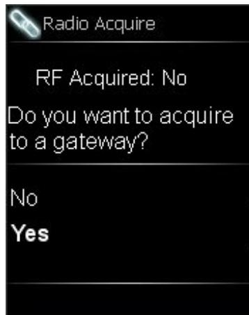
Before the MLX-3N can be used, it must first be acquired by a CEN-RFGW-EX gateway (sold separately) that is connected to an infiNET EX<sup>®</sup> system.
