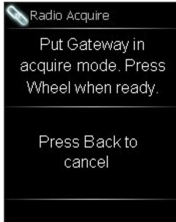
2. Put the CEN-RFGW-EX in *Acquire* mode by pressing its **ACQUIRE** button (on the unit itself or from Crestron Toolbox™, as described in the latest version of the CEN-RFGW-EX infiNET EX Gateway Operations & Installation Guide (Doc. 6706), which is available from the Crestron® Web site at [www.crestron.com/manuals](http://www.crestron.com/manuals)). The gateway’s **ACQUIRE** LED lights.
