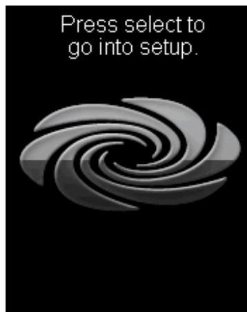
Press **SELECT** (or the scroll wheel) to display the “Setup Options” screen, as shown in the following illustration.
