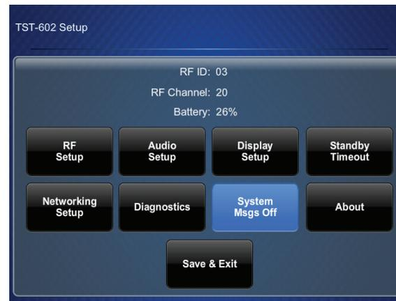
From the device's main setup screen, tap **RF Setup** to display the **RF Setup** screen.
