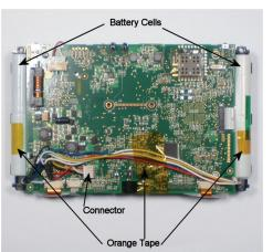
6. Carefully turn the assembly over returning it to its normal, face-up position. Then, place the assembly into the rear half of the TPS-6X enclosure, and hinge it so the top of the assembly is in place first (as shown in the following illustration). With the top of the assembly in position, settle the bottom of the assembly into place. Then, with your thumbs on the black plastic at the left and right edges, press and snap the assembly into place.
