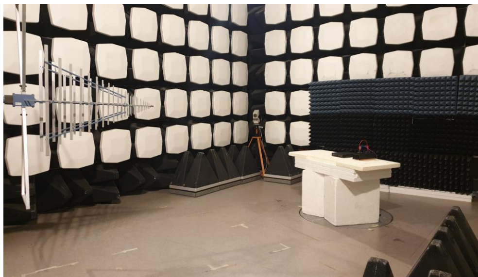
Photo 2. Radiated emission test setup for 30 - 1000 MHz.
