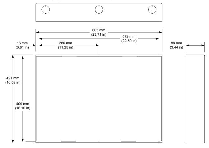
**NOTE:** Knockout holes are intended for Class 2 wiring only and are 38 mm (1 1/2") diameter.
