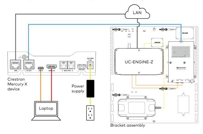
3. Connect the display devices and camera to components on the bracket assembly as shown below.
