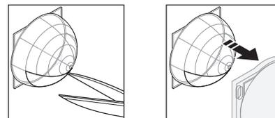
Shrouds supplied with each unit allow users to adjust coverage as needed.
