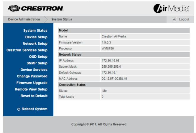
**NOTE:** Changes made in any section of the **Device Administration** menu require that the AM-100 be rebooted for the settings to take effect. For details, refer to "Reboot System" on page 22 for details.
