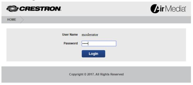
3. Enter the moderator password (the default password is "moderator") and click **Login**. The **Layout Control** screen is displayed showing a list of connected presenters.
