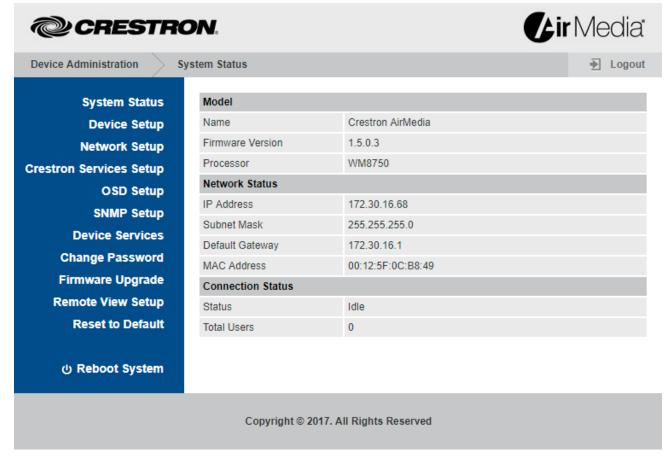
The **System Status** screen displays the device's name (hostname), firmware version, network status (IP address, subnet mask, default gateway, and MAC address), and connection status.
