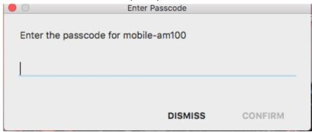
2. Enter the code displayed on the AM-100 welcome screen in the **Code** field and click **OK** (**CONFIRM** on Mac). The client establishes a connection between the computer and the AM-100 while displaying the Crestron AirMedia controls on the computer.
