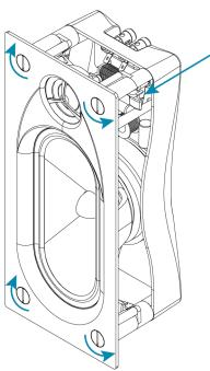
Spring Lock in unlocked position
