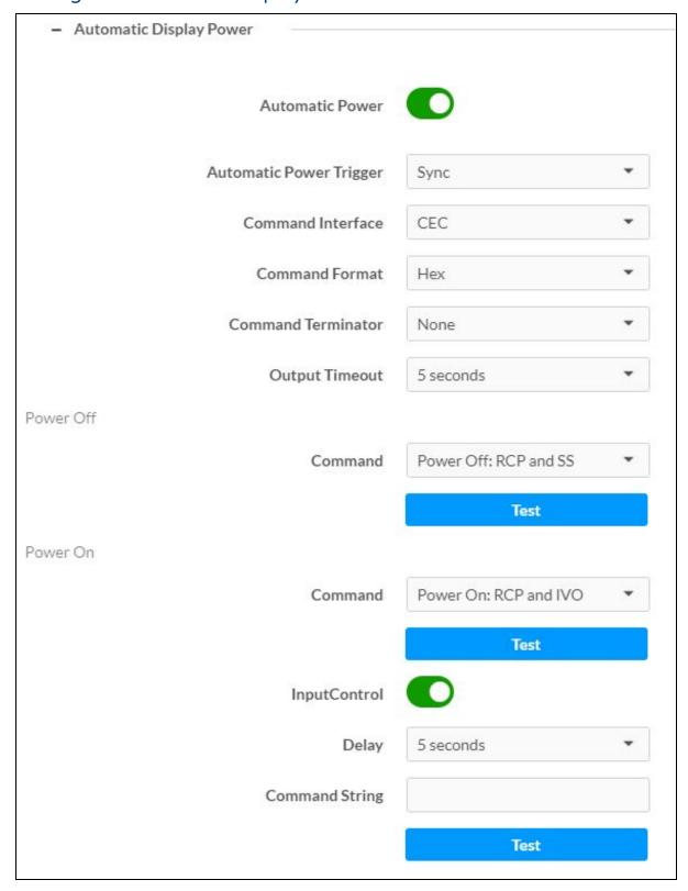
Move the **Automatic Power** slider to the right to enable automatic power. To disable, automatic power, move the slider to the left.
