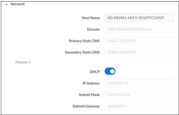
**NOTE:** By default the host name of the AV switchers consists of the model name followed by the MAC address of the device. For example, HD-MD4X1-4KZ-E-00107FCE6929.
