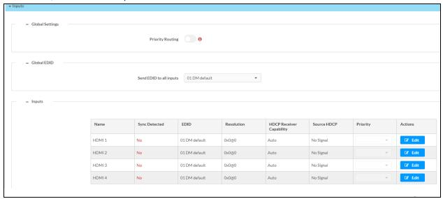
**NOTE:** Under the **Inputs** panel, the **Priority Routing** option is disabled. For Priority Routing to work, make sure that Auto Routing is enabled under the **Routing** panel.
