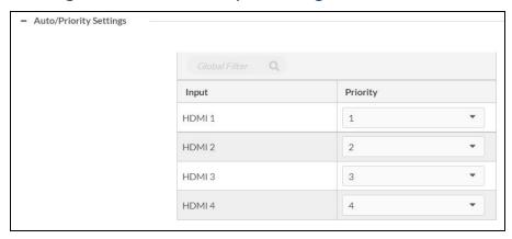
**NOTE:** For Priority Routing to work, make sure that Auto Routing is enabled under the **Routing** panel.
