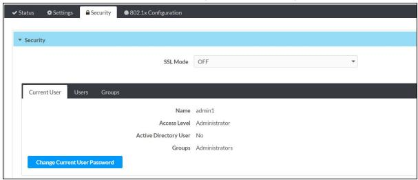
Select **Encrypt and Validate**, **Encrypt**, or **OFF** in the **SSL Mode** drop-down menu, to specify whether to use encryption. By default SSL Mode is set to OFF.
