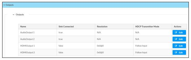
The Outputs section displays information and allows settings to be modified for available outputs.
