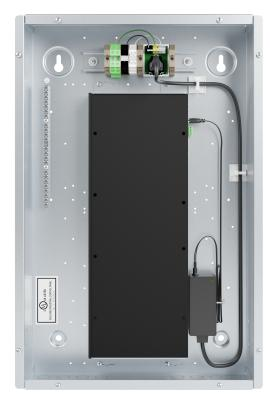
The Crestron® ZUML-HUB4 is a preassembled lighting control cabinet for use with a Crestron Zūm® lighting system. It contains a ZUM-HUB4 Zūm hub and PW-2420RU power pack mounted in a DIN-EN-3X18 wall mount enclosure. It provides a convenient solution for networked commercial lighting applications.
