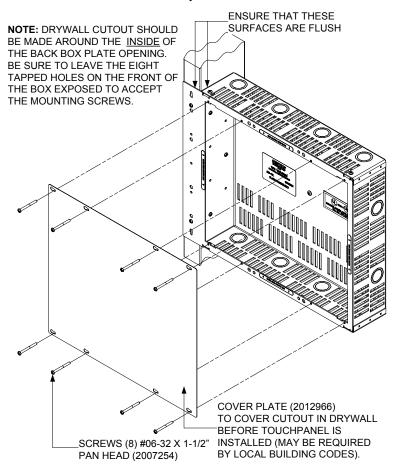
**NOTE:** Cut the drywall along the inside edge of the front of the back box. The labels on the front of the back box indicate the perimeter of the opening that should be cutout. Refer to the **NOTE** in "Mounting the Back Box" shown on previous page.
