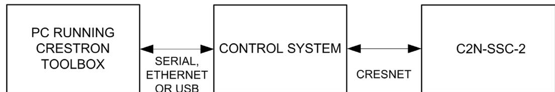
C2N-SSC-2 connects to control system via Cresnet:
