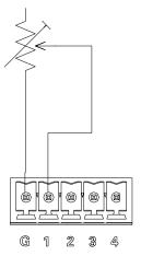
I/O Setup: Analog Input
