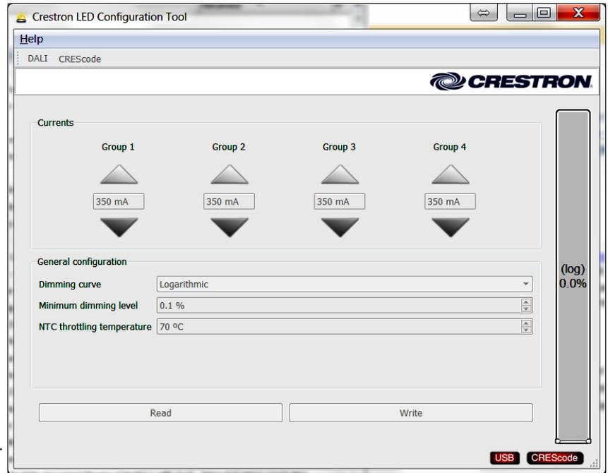
To save your new settings to the driver for Dimming curve, Minimum dimming level and NTC temperature, press the Write button.
