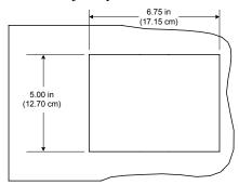
If the opening is too large, two pre-construction accessories are available to make adjustments. Use the optional TMK-6L (Trim Ring Kit) to provide a smooth edge at the opening. This option provides a finished appearance and is preferred with wallpaper. Use the optional MMK-6L (Mud Ring Kit) to fill in larger irregularities around the opening (requires plastering).
