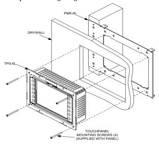
CAUTION: Allow an air gap of at least 12 inches in the wall cavity above and below the touchpanel for heat dissipation.
