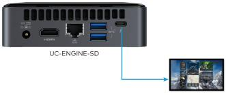
Connect the CBL-USBC-HD-9 to the USB-C port on the UC-ENGINE-SD and to the display.
