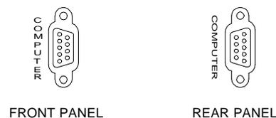
These 9-pin DB9 female connectors (one on the front panel and one on the CNXCPU) are used when programming with a PC. A standard DB9 female (PC end) to DB9 male (CNRACKX end) straight-through serial cable (not supplied) is used to communicate with either COMPUTER port. The ports are electrically connected and are modem compatible. The modem cable is not included.
